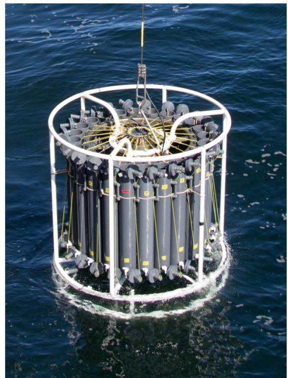
**Fig. 1:** CTD device in operation.
